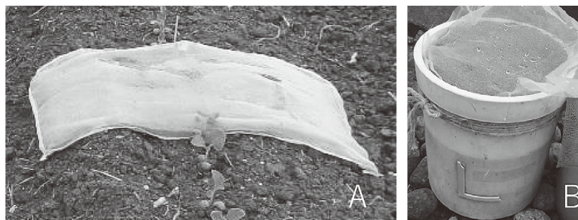
Fig. 1 Rectangular sandbag trap (A) and a circle sandbag trap (B)
